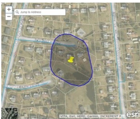
Esri map as seen on SOSRemote device. The area to be marked can be highlighted based on geo coordinates in the 811 notification.
